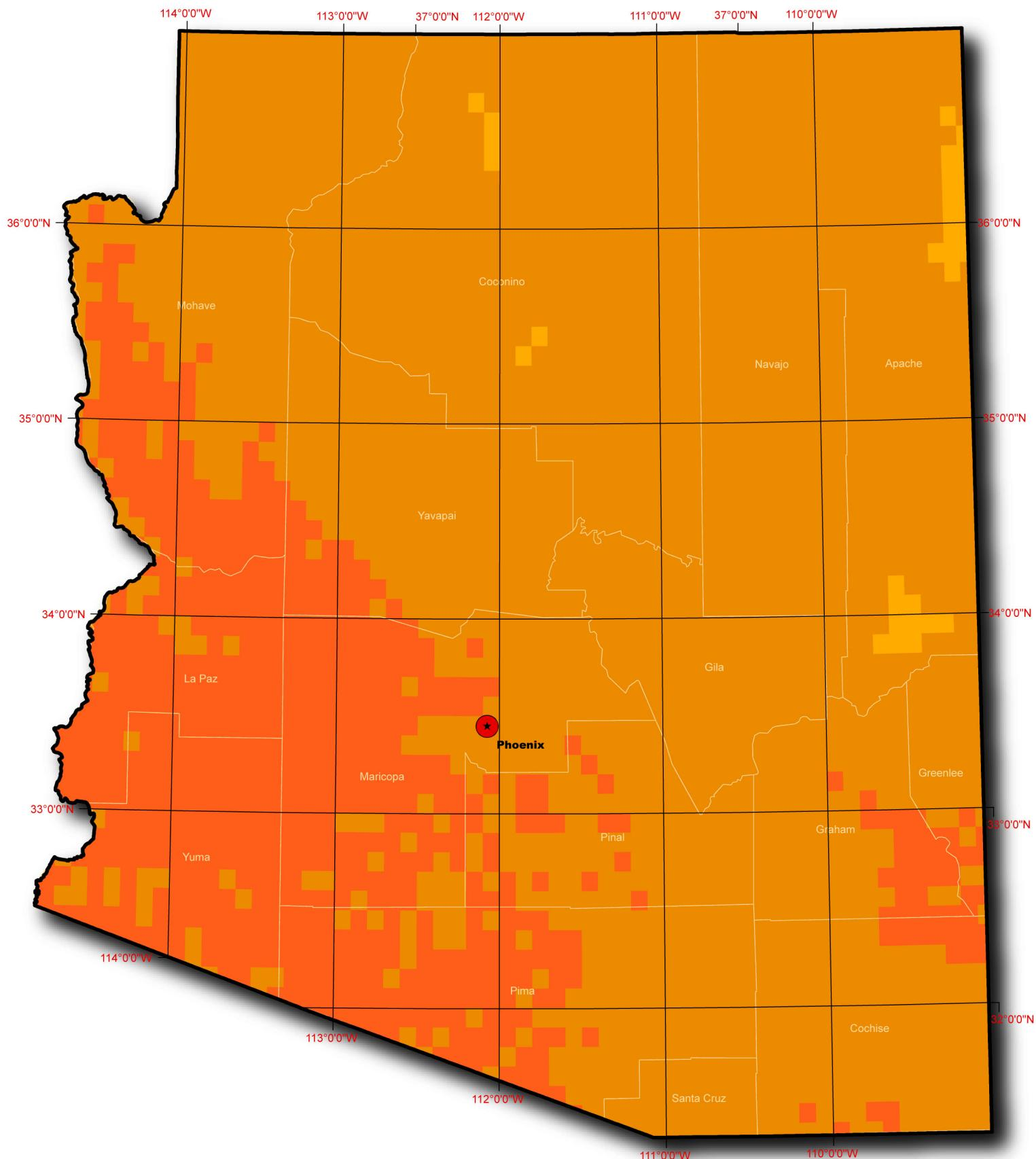
Model estimates of monthly average daily total radiation, averaged from hourly estimates of direct normal irradiance over 8 years (1998-2005). The model inputs are hourly visible irradiance from the GOES geostationary satellites, and monthly average aerosol optical depth, precipitable water vapor, and ozone sampled at a 10km resolution.
